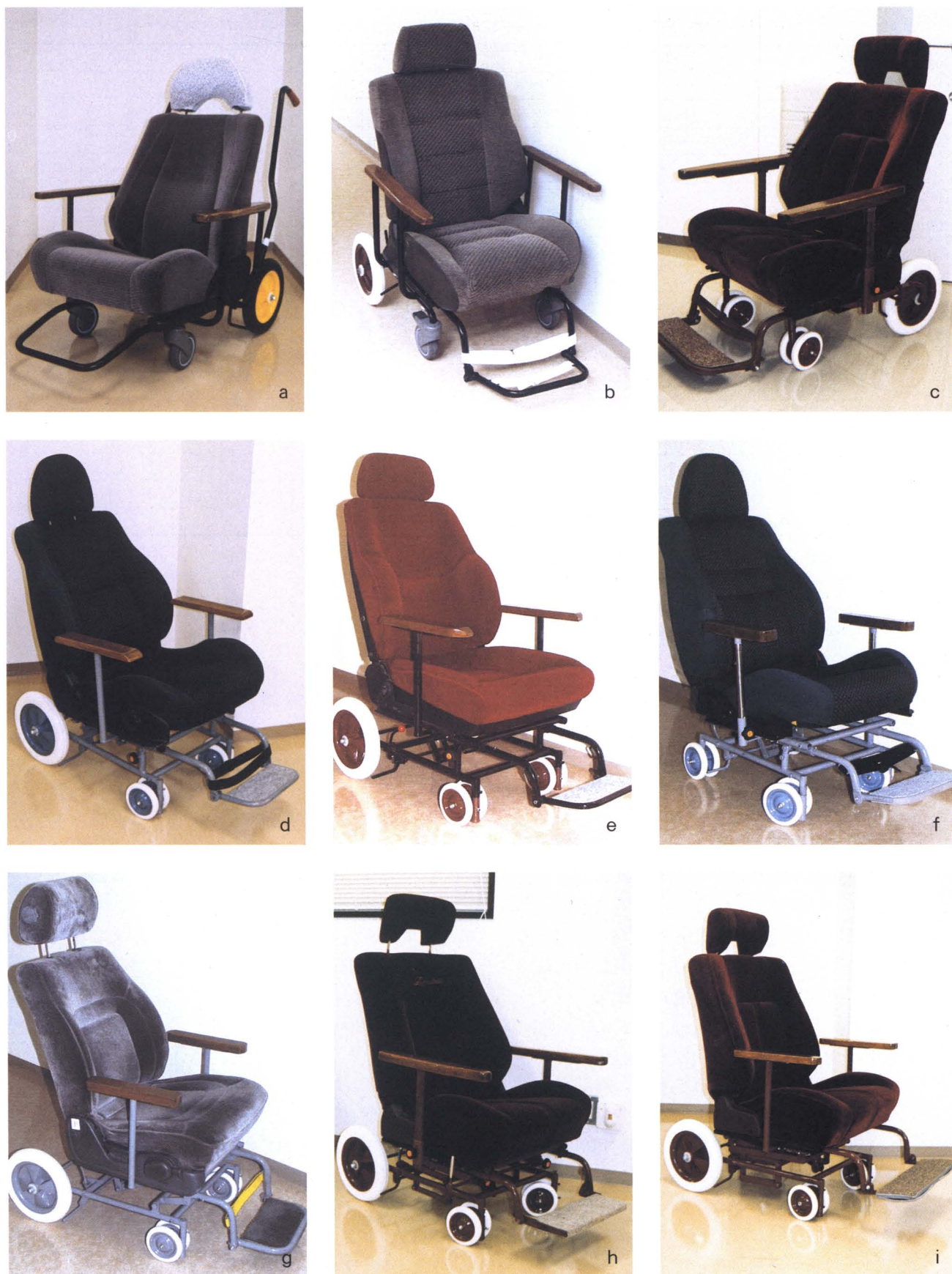
Figure 2. Photographs of wheelchairs made by reuse of car seat. (a) Model A, (b) model B, (c) model C, (d) model D, (e) model E, (f) model F, (g) model G, (h) model H, (i) model I.
